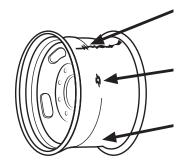
Leak at butt weld caused by cracked or damaged weld.
